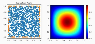
**Figure 8:** The figures shows on the left the points used to evaluate the collocation error, while the right one can see the solution at inference time on million degree of freedom.
