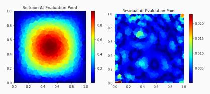
**Figure 7:** The figures above show the first eigenfunction of the Laplacian computed numerically and the residual both in the collocation points.
