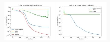
**Figure 3:** The figure show how the objective function decays for four different method Newton, Gauss-Newton, BFGS and ADAM.
